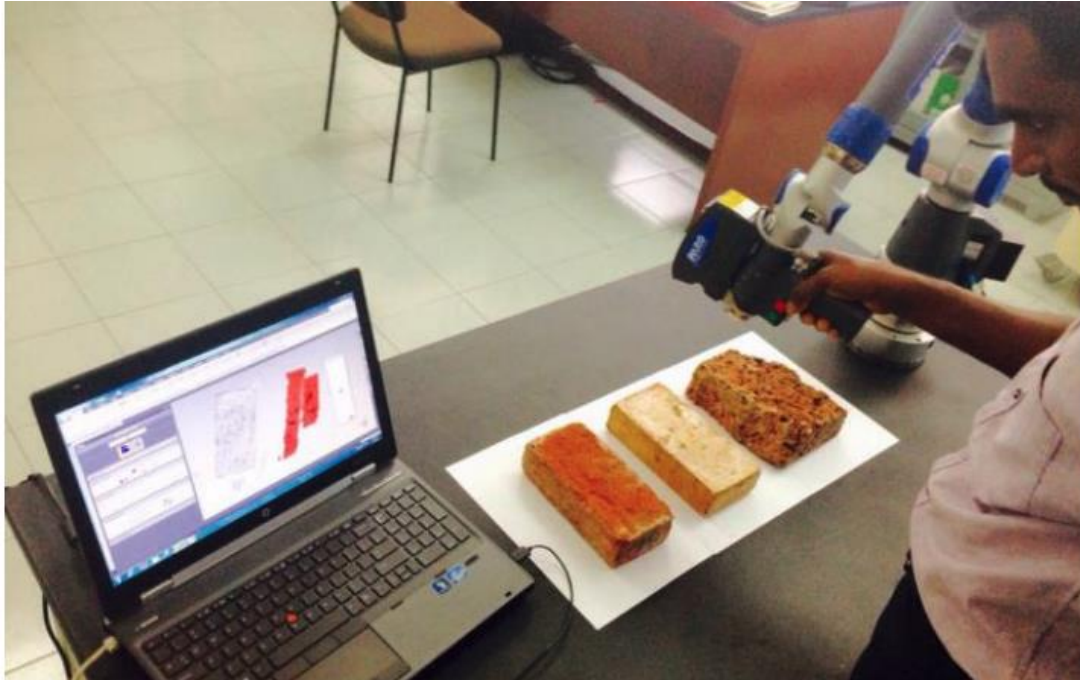
Figure 34. A researcher scanning the surface complexity of different building materials. Source: Udawattha et al., 2018.
