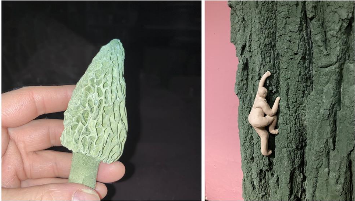
Figure 33. Cement casts of natural objects with high surface complexity. (Left) cast of a black morel mushroom ( Morchella elata ); (right) cast of especially furrowed bark with a sculpted figure. The cement used for these casts was modified with sawdust and wood mould to enhance bio-receptivity. Source: RJH Artworks, 2022.
